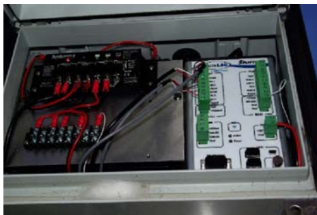
Figure 2 Internal connection between the H-377 temperature sensor probes and STORM 3 Data Logger (see online version for colours)
