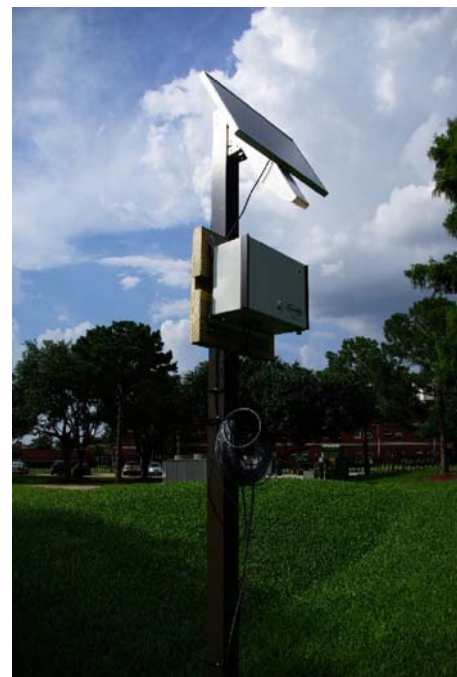
Figure 6 Deployment of STORM 3 Data Logger and H-377 Temperature Probe to monitor the pond close to John Gray Center at Lamar University, Beaumont, TX (see online version for colours)
