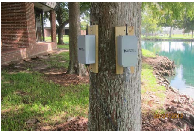
Figure 10 Deployment of NI Wireless Modules and DO and pH Sensors around the pond close to John Gray Center at Lamar University, Beaumont, TX (see online version for colours)
